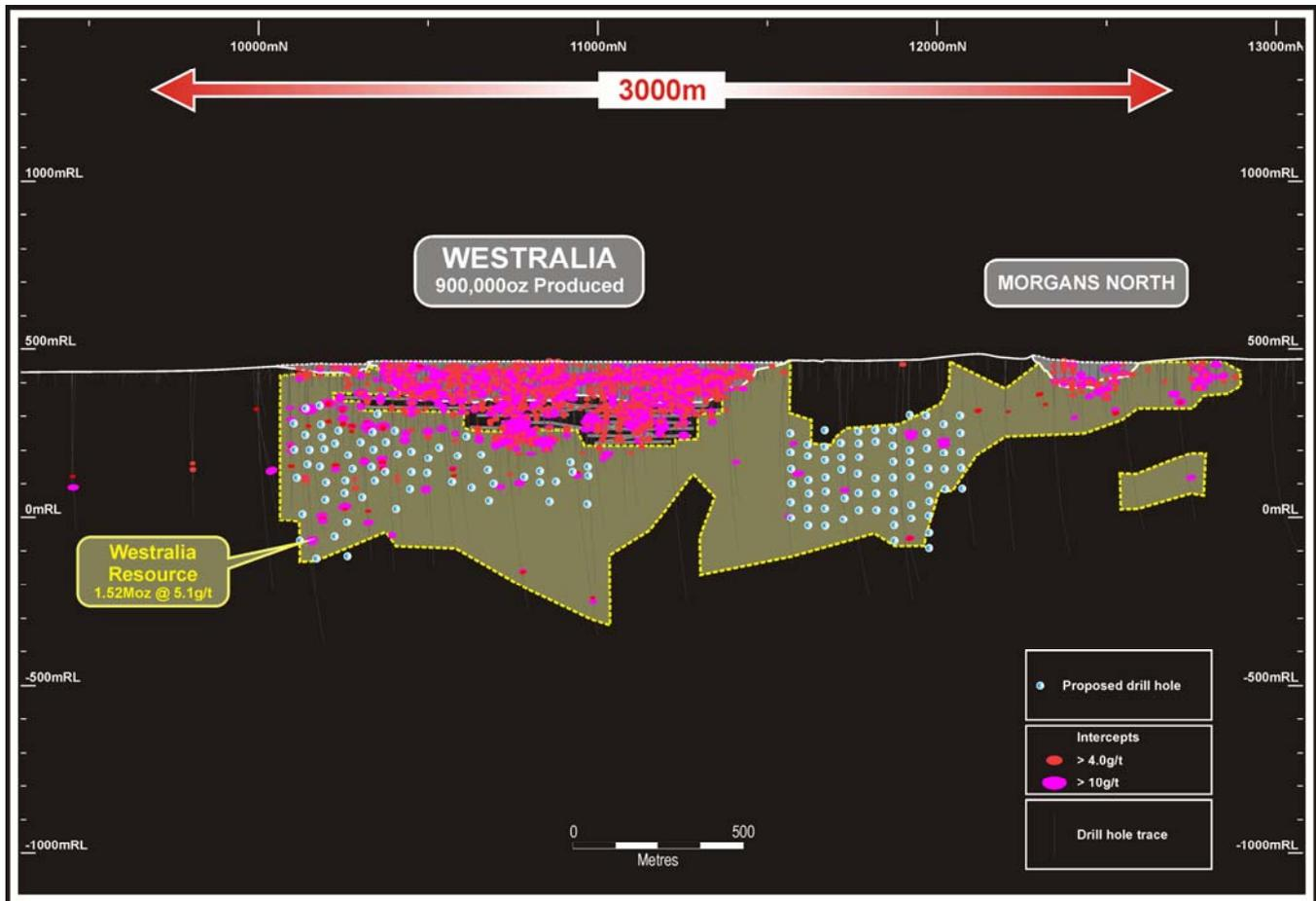
**Figure 1:** Planned drilling program over the Westralia Prospect with 62 diamond drill holes planned for potential Westralia Underground (blue dots on left hand side of image) and 67 diamond drill holes planned for potential Morgans Underground (blue dots on right hand side of image).
