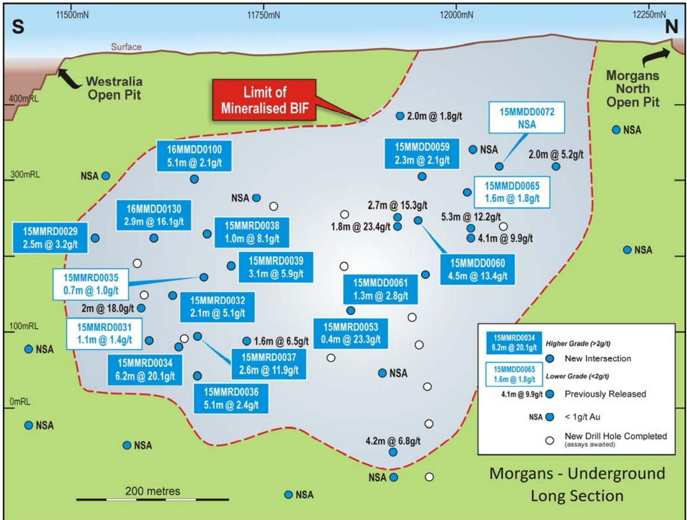
**Figure 2:** Long section of the potential Morgans Underground mineralisation measuring 700m long and up to 400m in dip (or vertical) extent. New high grade intersections are shown in blue boxes and existing intersections are shown without boxes. The location of the 13 holes that have been drilled and have assays awaited are shown as white circles.
