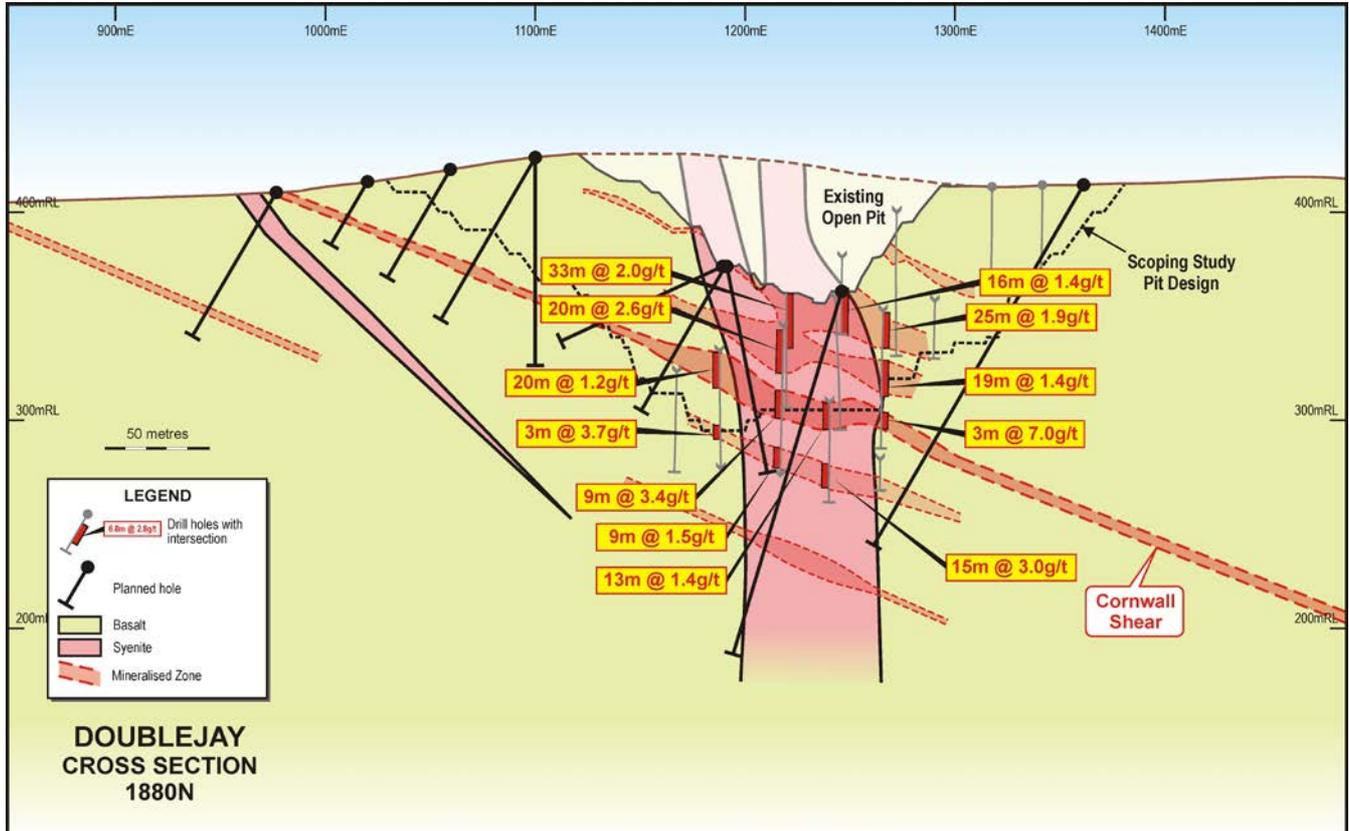
**Figure 4:** Cross Section 1880N through the Doublejay open pit showing the existing pit excavation, the Scoping Study Pit design and the planned drilling (bold black lines). The southern section of the historic open pit did not mine the Cornwall Shear Zone where there are significant unmined intersections below the existing pit floor. Note the extensive hangingwall and footwall mineralisation above and below the CSZ (also mineralised) and lack of testing of the CSZ up-dip in basalt.
