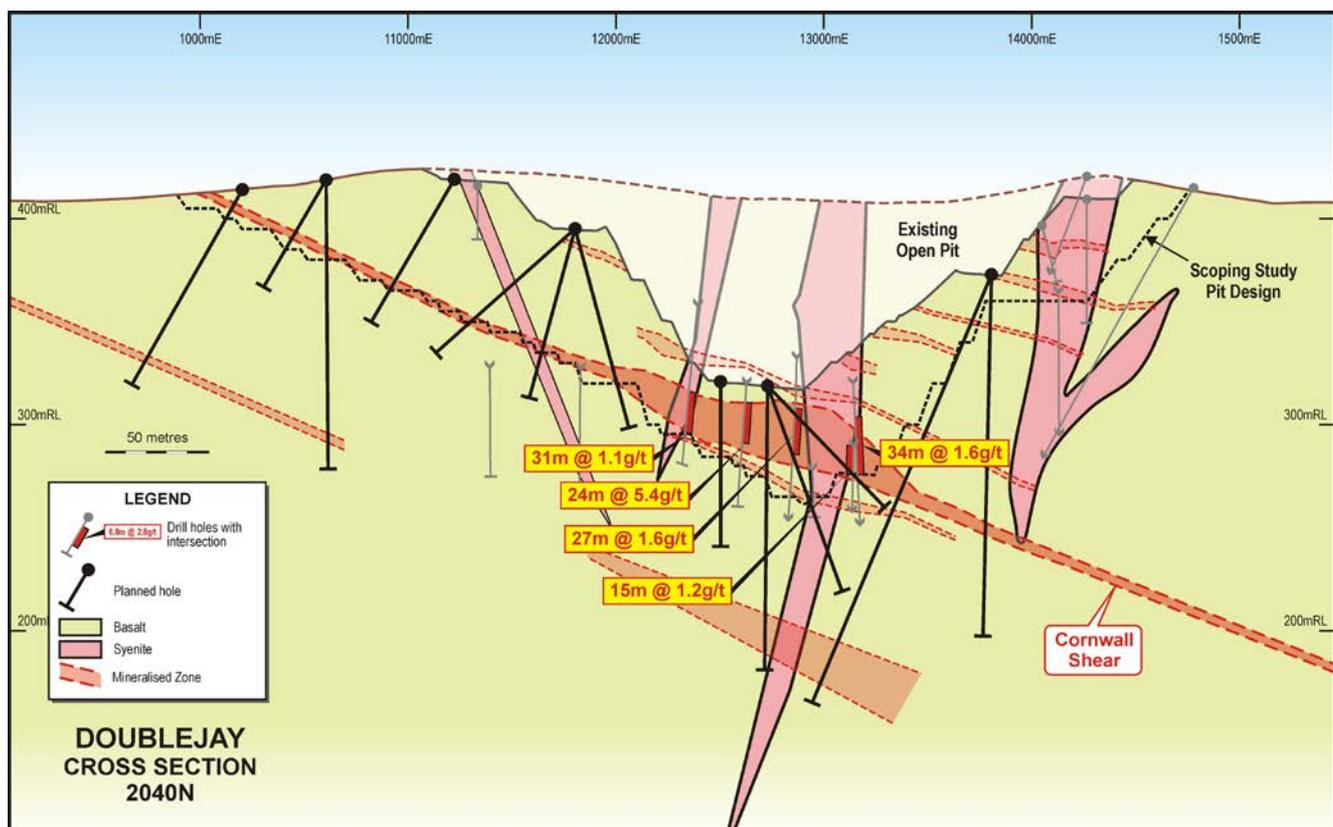
**Figure 3:** Cross Section 2040N through the Doublejay open pit. Note the existing pit excavation, the Scoping Study design shell and the planned drilling (bold black lines). There are several significant intersections of the CSZ below the base of the existing open pit including 24m at 5.4g/t Au, 34m @ 1.6 g/t Au and 27m @ 1.6 g/t Au.
