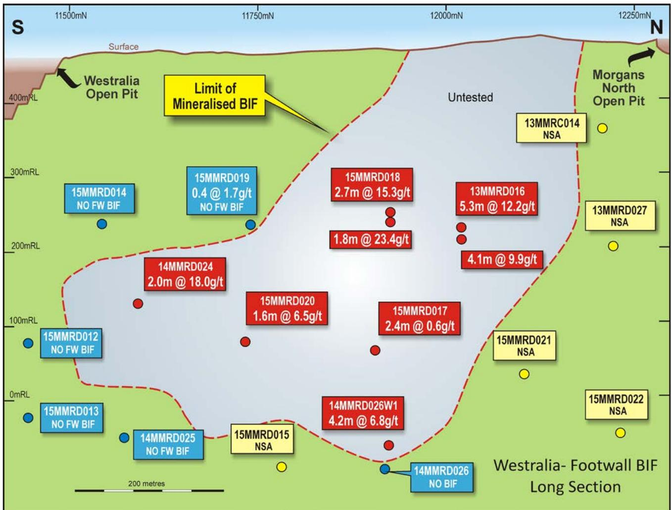
**Figure 2:** Long section of the newly discovered footwall BIF unit located between the Westralia and Morgan North open pits. Note the broad spacing of the mineralised intersections is approximately 200m x 200m; and the up-dip expression of the mineralised footwall BIF unit toward the surface is untested.
