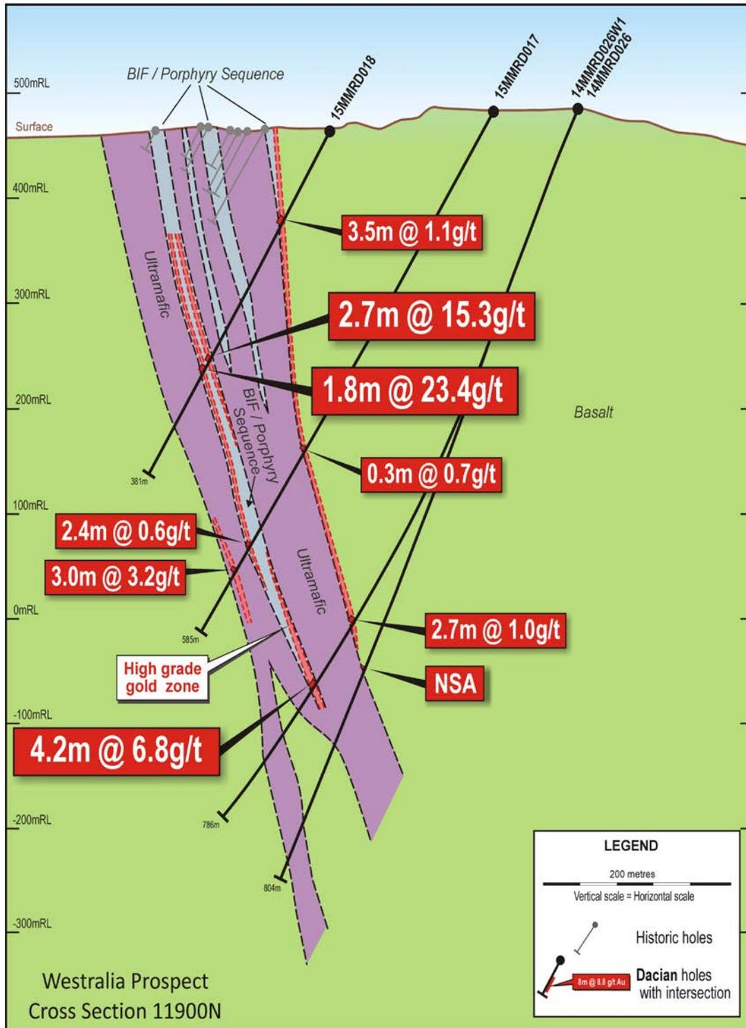
**Figure 3:** Section 11900N showing high grade mineralisation in the newly identified footwall BIF. Note the 400m dip-extent of mineralisation identified between drill holes 15MMRD018 and 14MMRD026W1.
