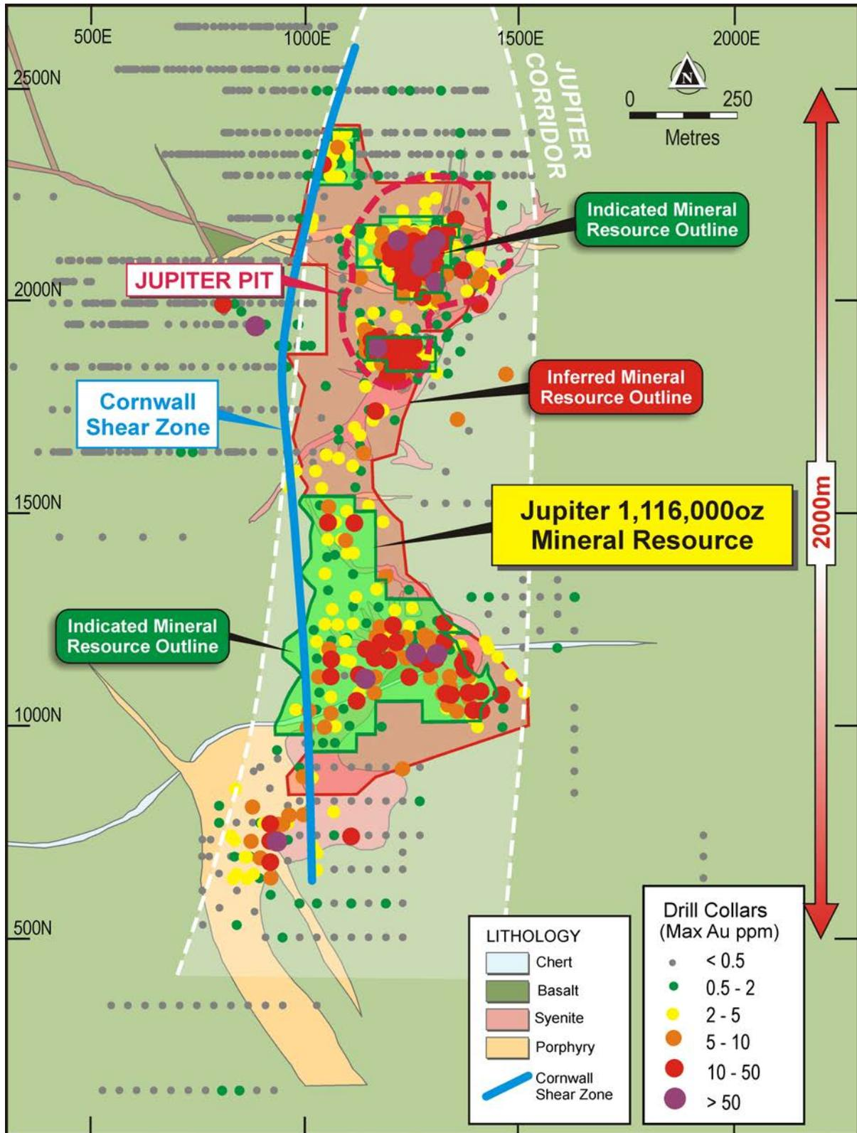
**Figure 5:** Local geological setting of the Jupiter Prospect. Note the north–south alignment of the Jupiter Corridor and the Cornwall Shear Zone. The Jupiter Prospect Mineral Resource is shown in plan view and colour-coded green for Indicated Resource and red for Inferred Resource.
