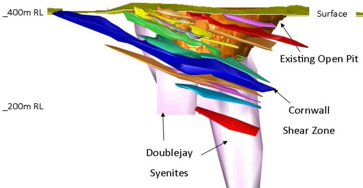
**Figure 3:** Isometric cross-sectional view (looking north) of the high grade lodes developed within in the Doublejay syenite (light purple colour) and outside the historic Jupiter open pit. The dominantly mineralised Cornwall Shear Zone which outcrops to the west (left hand side of image) is coloured blue.
