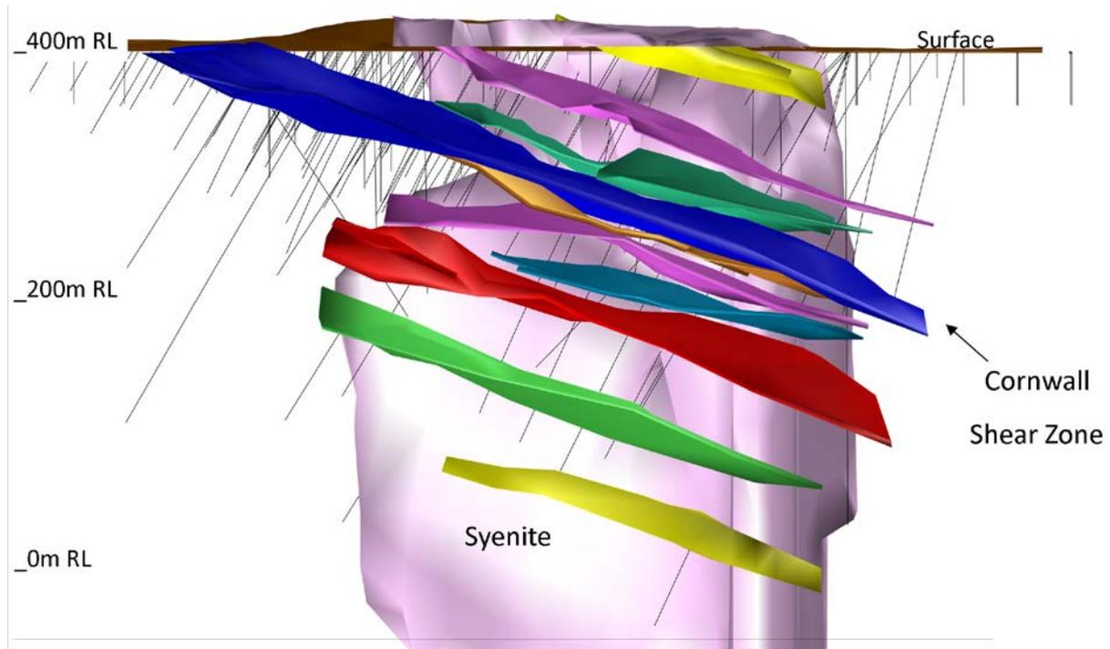
**Figure 4:** Isometric cross-sectional view (looking north) of the high grade lodes developed principally in the Heffernans syenite (light purple colour) and associated drilling. The dominantly mineralised Cornwall Shear Zone which outcrops to the west (left hand side of image) is coloured blue.
